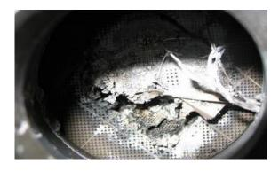
For particulate filters which have mechanical damage such as fusion through overheating, the particulate filter must be replaced
