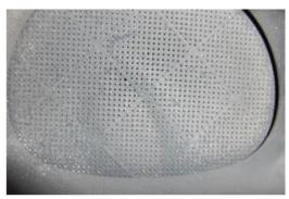
If the particulate filter is clogged as in this example, this can be cleaned with the TUNAP system.
