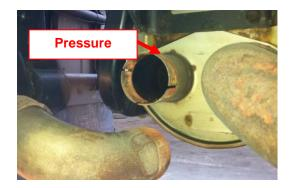
1. Remove the pressure sensor or disconnect the filter from exhaust pipe.
