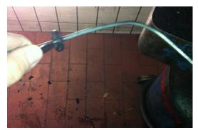
Insert the spraying probe into the opening made with the direction of spraying towards the particulate filter. Bend the probe slightly if necessary
